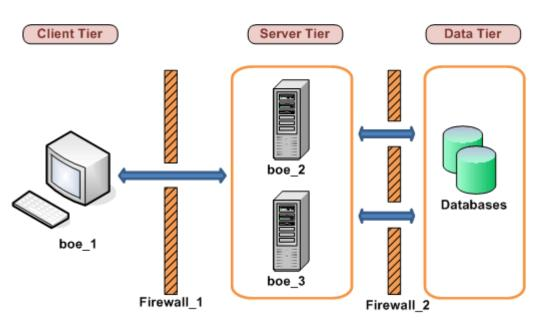
Figure 11: Rich client and database tier deployed on separate networks
